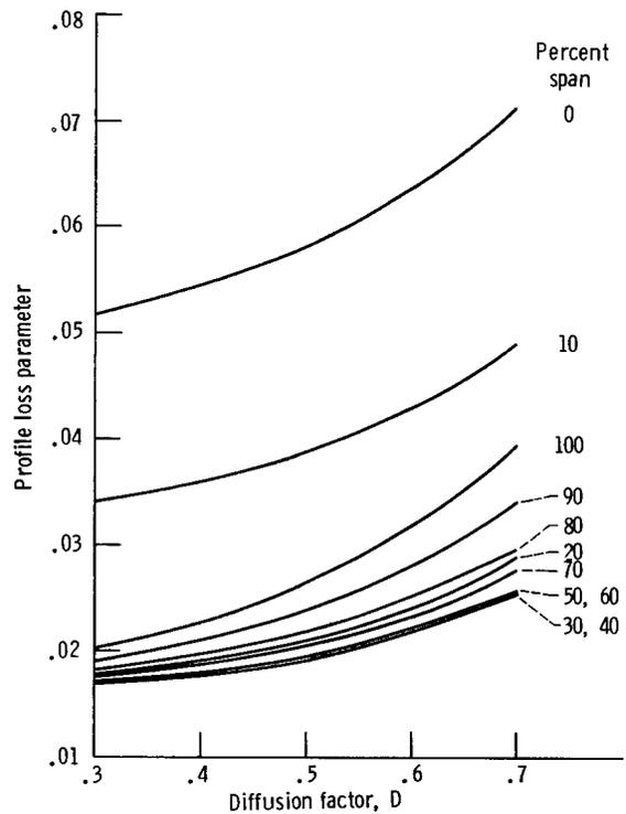
Figure 7.—Stator profile losses. (See eqs. (B13) and (B21).)
