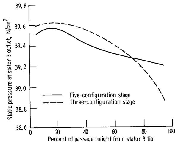
Figure 3.—Design static pressures at stator 3 trailing edge.
