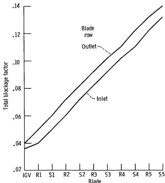
Figure 4.—Total blockage factors applied to flowpath.
