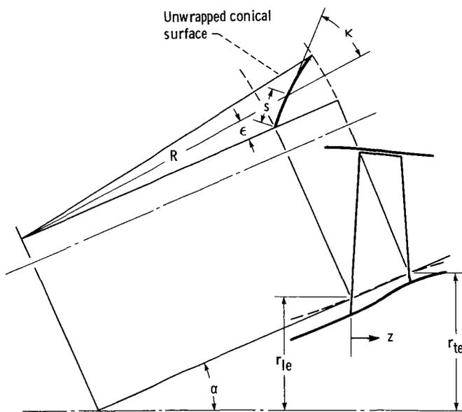
Figure 9.—Conical coordinate system for blade-element layout.
