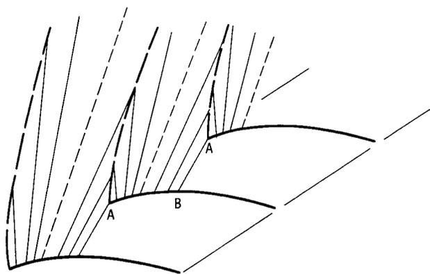
Figure 11.—Extended wave pattern ahead of supersonic cascade with curved entrance region AB.
