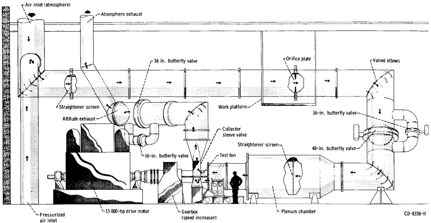
Figure 17.—Multistage compressor test facility.
