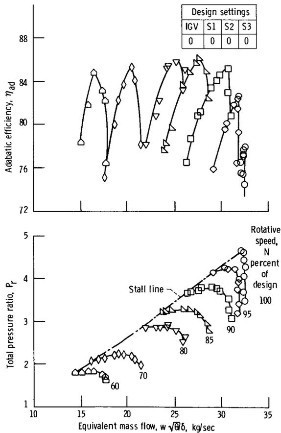
Figure 18.—Performance of first three stages of compressor 74A at design IGV-stator setting angles.
