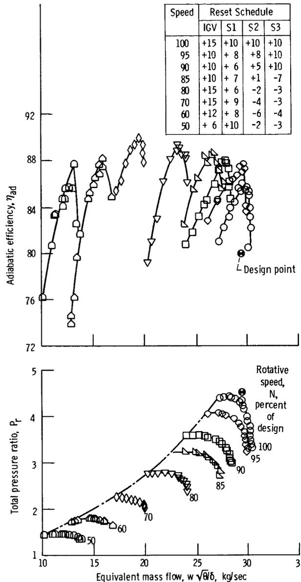
Figure 22.—Performance of first three stages of compressor 74A at optimized IGV-stator setting angles for maximum efficiency at each speed shown.
