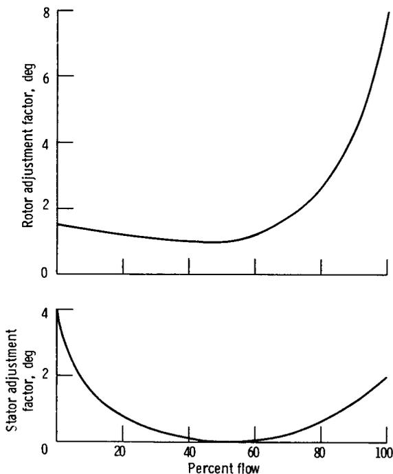
Figure 12.—Deviation adjustment factors added to Carter's rule.
