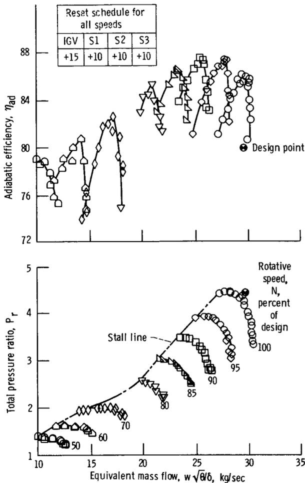
Figure 21.—Performance of first three stages of compressor 74A at optimized IGV-stator setting angles for maximum efficiency at design speed.
