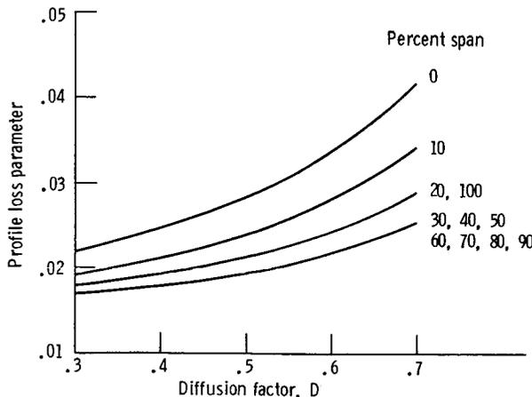
Figure 6.—Rotor profile losses. (See eqs. (B13) and (B21).)
