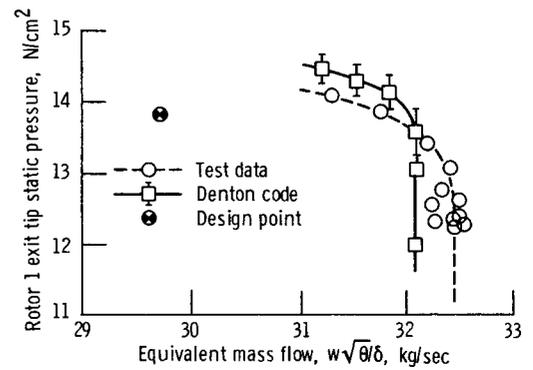
Figure 19.—Comparison of measured and computed rotor 1 exit tip static pressure versus mass flow.
