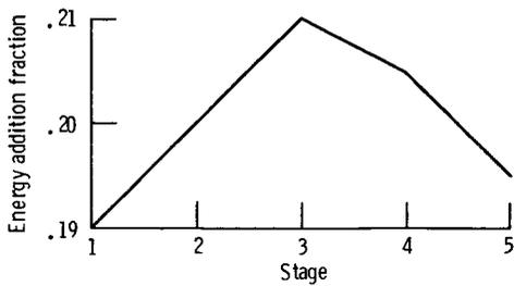
Figure 5.—Axial energy addition fraction per stage.
