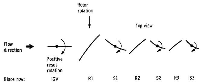
Figure 20.—Schematic of blade rows with positive direction of vane reset specified.
