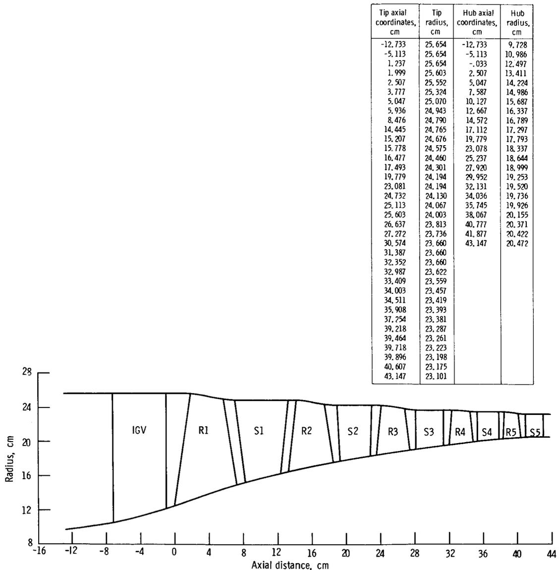
Figure 1.—Flowpath for compressor 74A.
