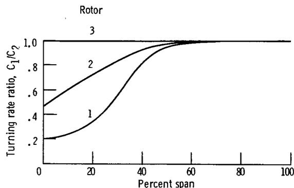
Figure 13.—Rotor blade element turning rate ratio.
