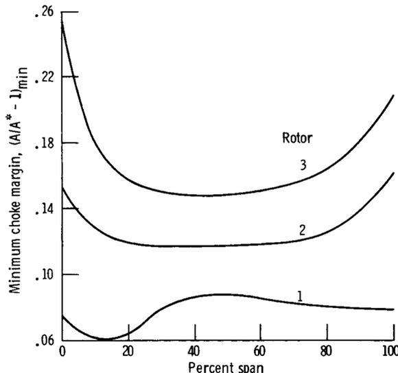
Figure 14.—Rotor blade element choke margin.
