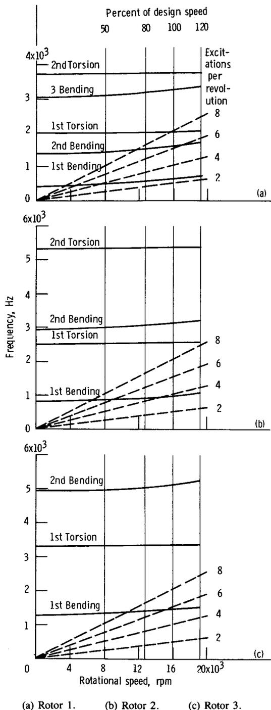
Figure 16.—Campbell diagrams for rotors.
