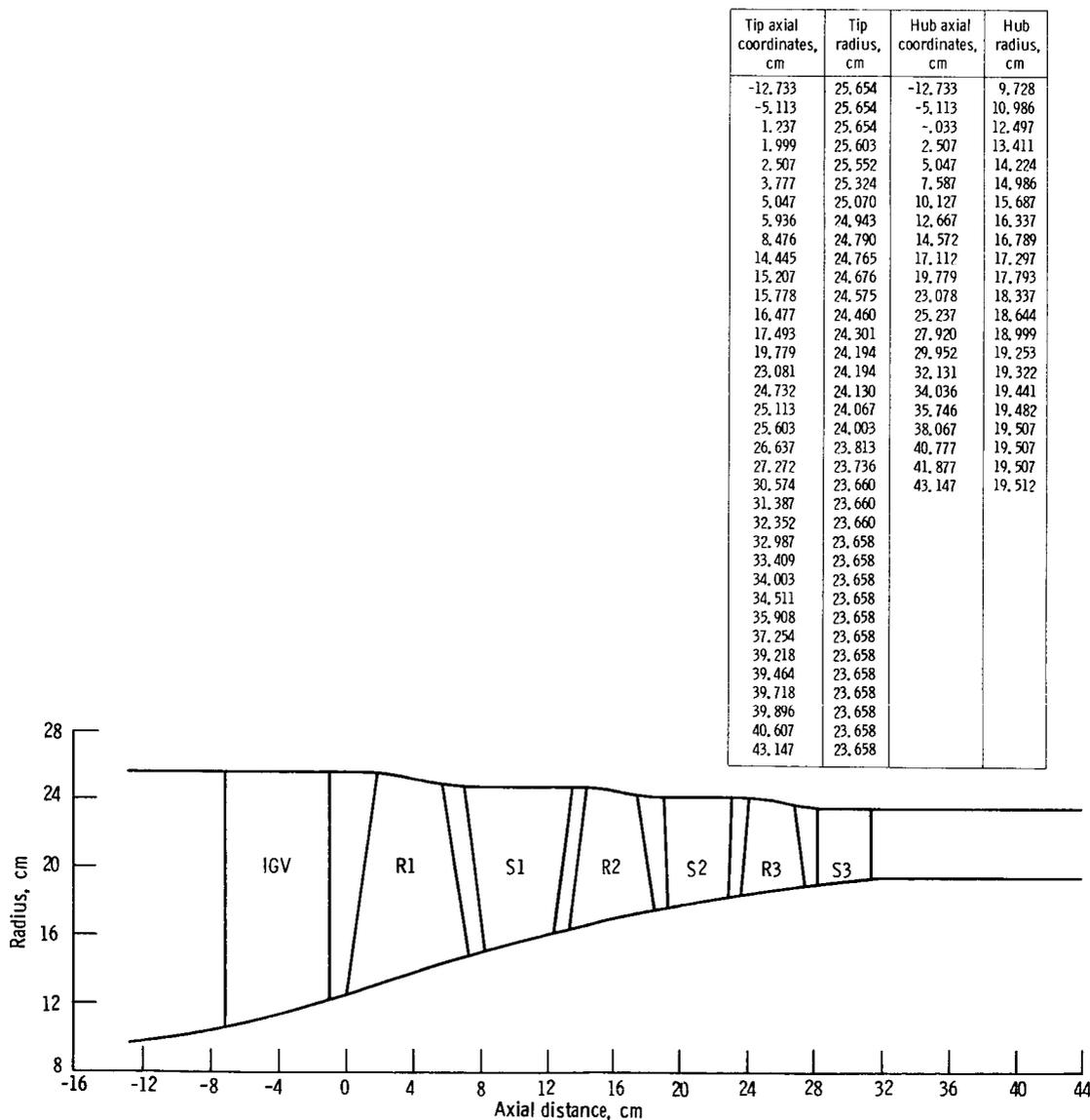
Figure 2.—Flowpath for inlet stage group of compressor 74A.
