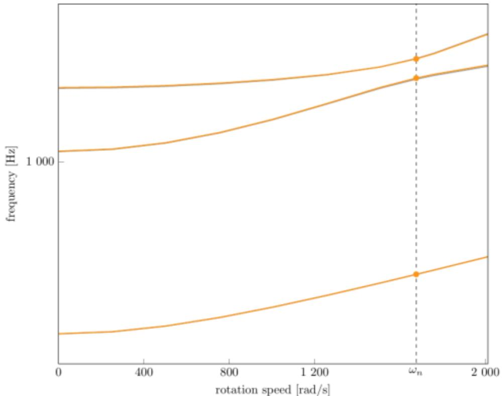
Campbell diagram computed with a linear centrifugal preload, with clamped root (nominal speed  $\omega_n = 1675.52$  rad/s),
