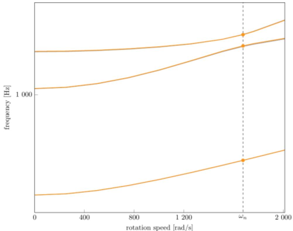
Campbell diagram computed with a linear centrifugal preload, with clamped root (nominal speed  $\omega_n = 1675.52 \text{ rad/s}$ ),
