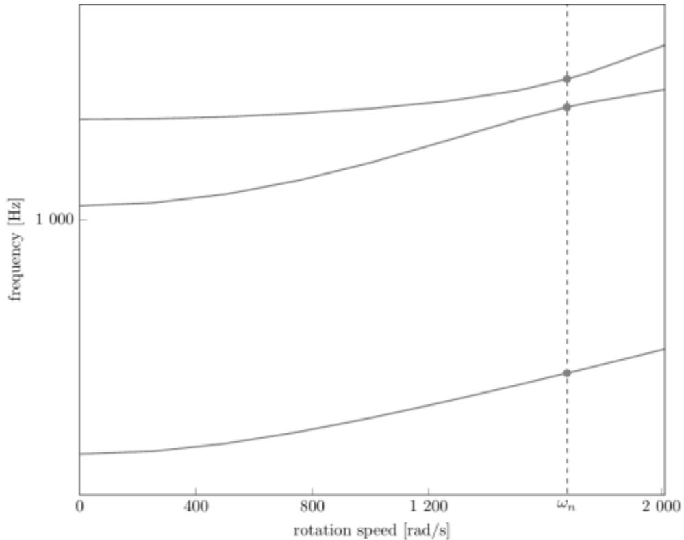
Campbell diagram computed with a linear centrifugal preload, with clamped root (nominal rotation speed  $\omega_n = 1675.52 \text{ rad/s}$ )
