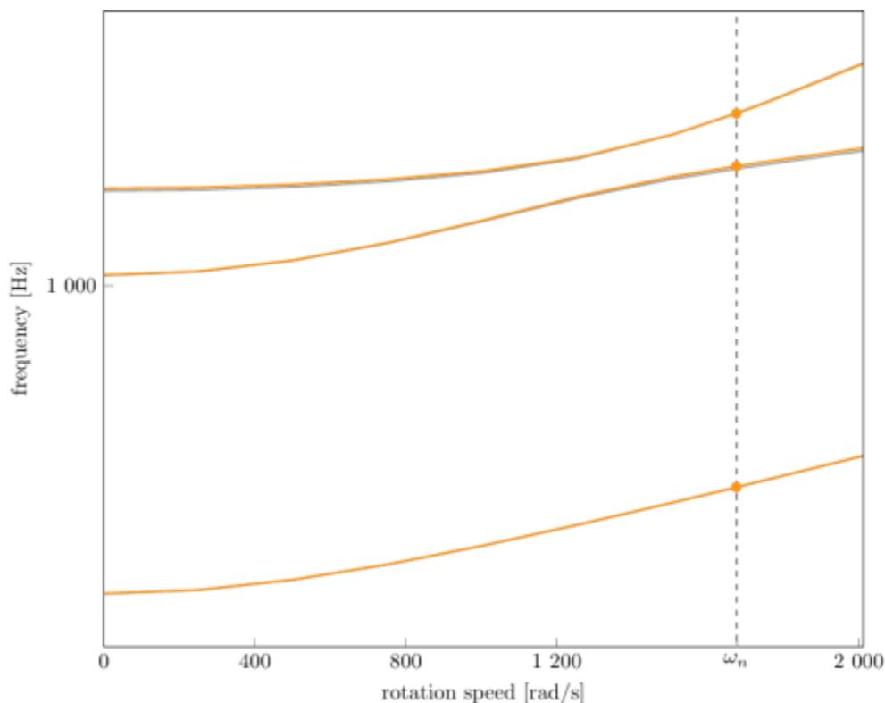
Campbell diagram computed with a linear centrifugal preload, with clamped root (nominal speed  $\omega_n = 1\ 675.51$  rad/s),
