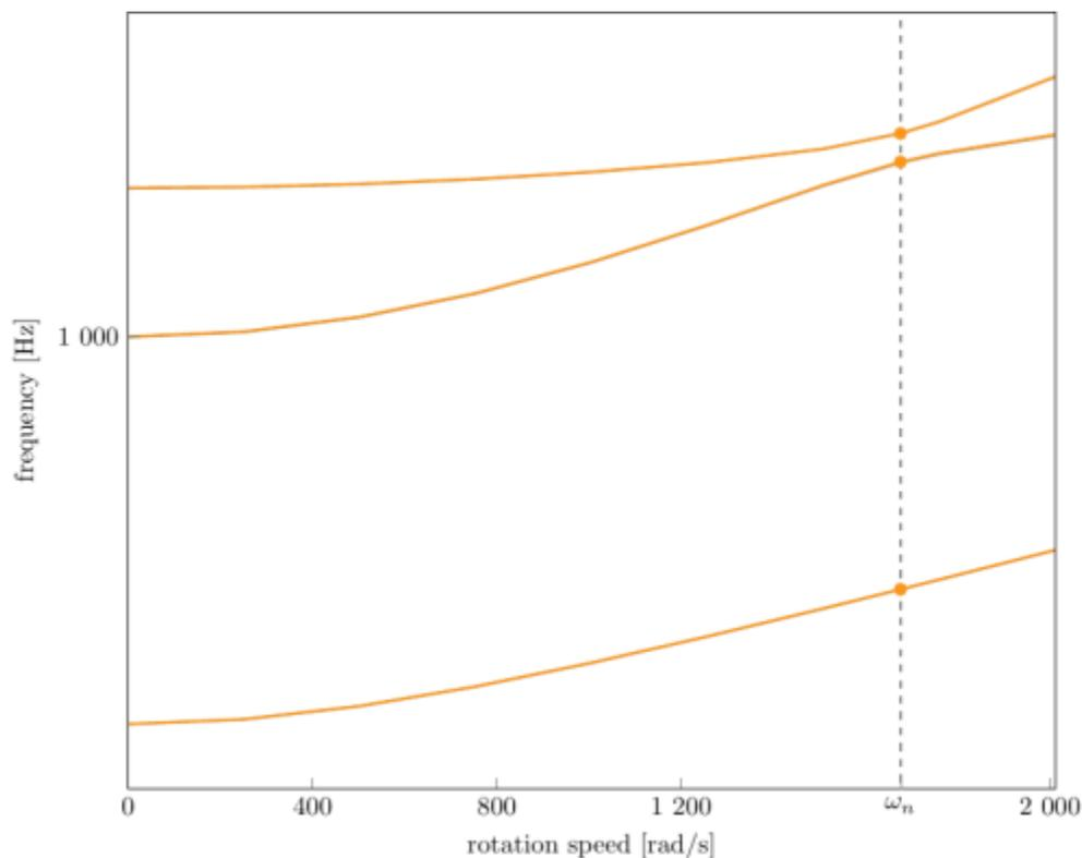
Campbell diagram computed with a linear centrifugal preload, with clamped root (nominal speed  $\omega_n = 1800$  rad/s),
