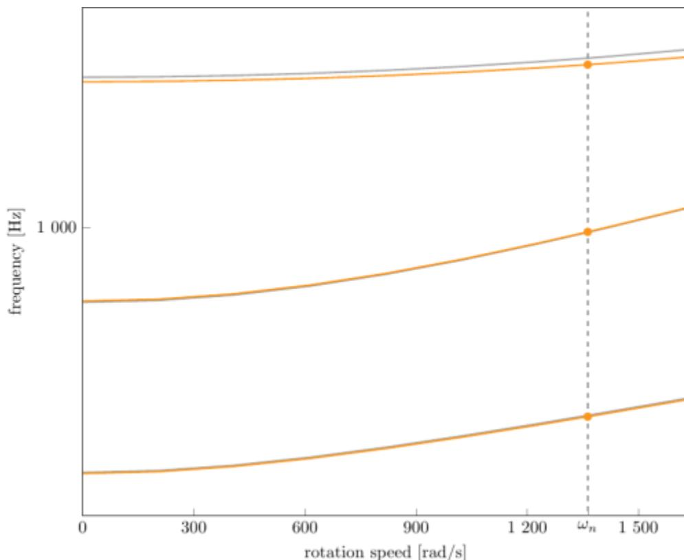
Campbell diagram computed with a linear centrifugal preload, with clamped root (nominal speed  $\omega_n = 1363.45$  rad/s),
