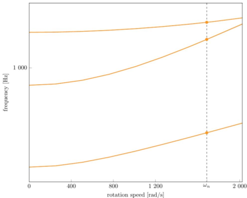
Campbell diagram computed with a linear centrifugal preload, with clamped root (nominal speed  $\omega_n = 1686$  rad/s),
