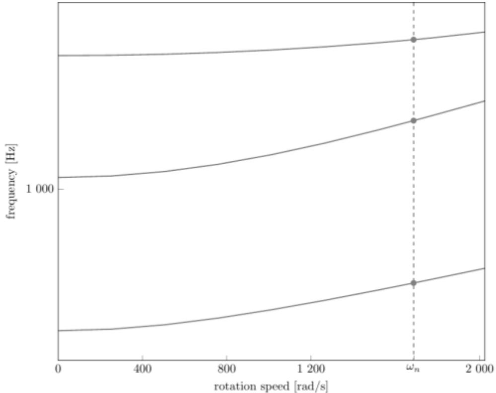
Campbell diagram computed with a linear centrifugal preload, with clamped root (nominal rotation speed  $\omega_n = 1\,686 \text{ rad/s}$ )
