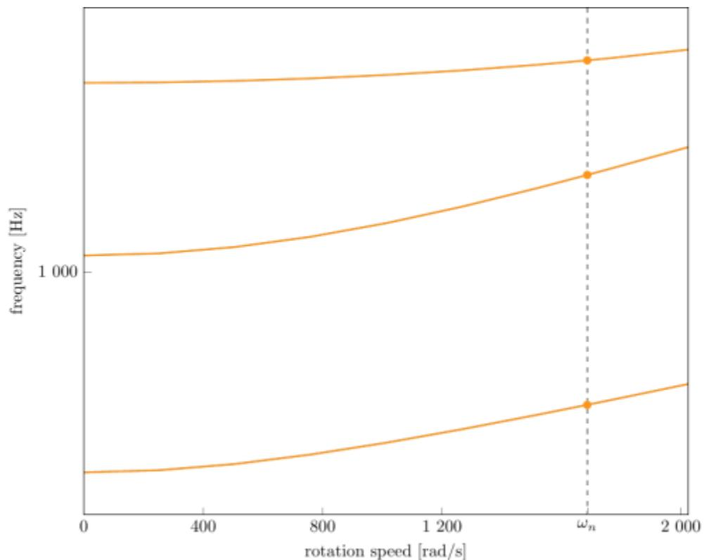
Campbell diagram computed with a linear centrifugal preload, with clamped root (nominal speed  $\omega_n = 1686$  rad/s),
