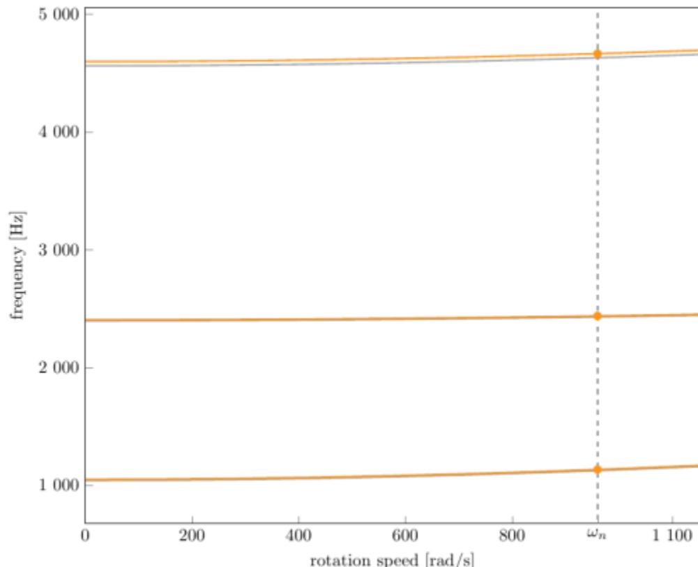
Campbell diagram computed with a linear centrifugal preload, with clamped root (nominal speed  $\omega_n = 960.28 \text{ rad/s}$ ),
