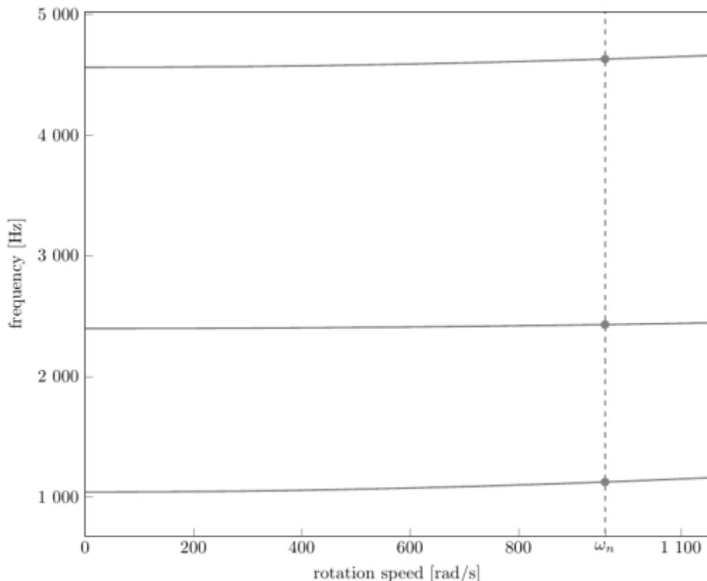
Campbell diagram computed with a linear centrifugal preload, with clamped root (nominal rotation speed  $\omega_n = 960.28 \text{ rad/s}$ )
