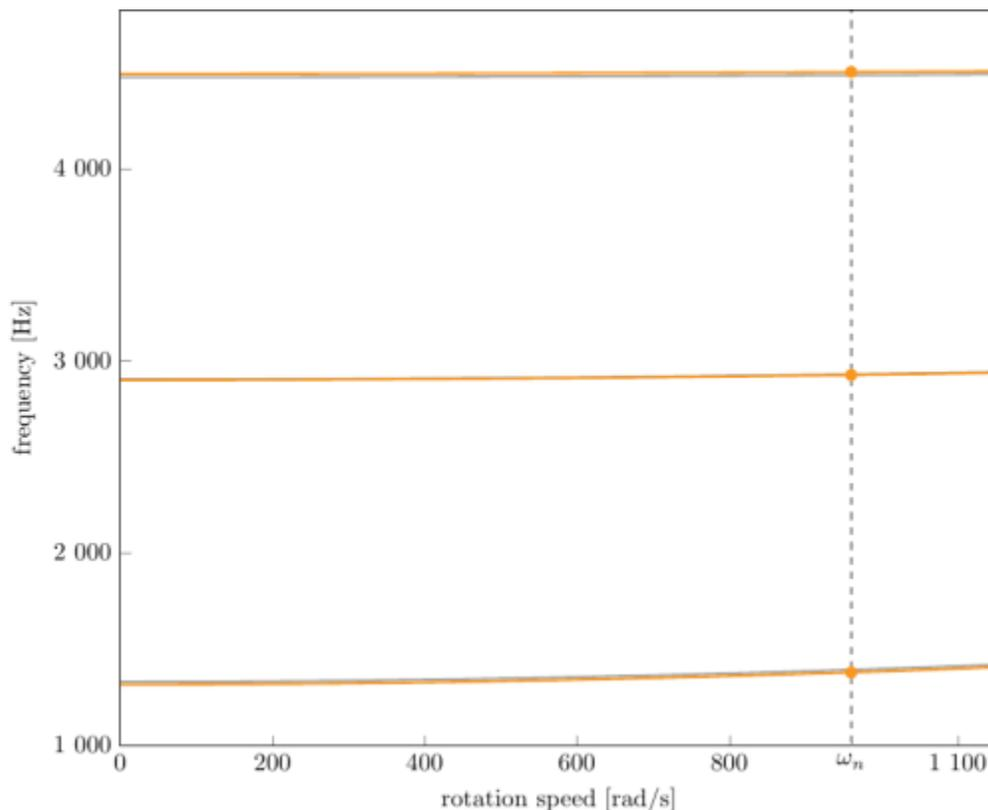
Campbell diagram computed with a linear centrifugal preload, with clamped root (nominal speed  $\omega_n = 960,28$  rad/s),
