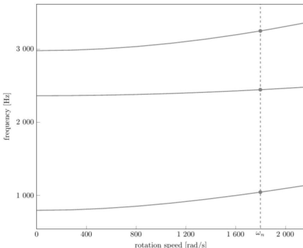
Campbell diagram computed with a linear centrifugal preload, with clamped root (nominal speed  $\omega_n = 1800$  rad/s),
