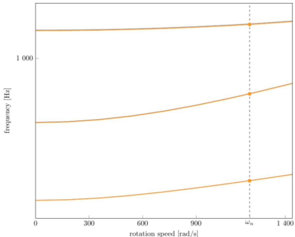
Campbell diagram computed with a linear centrifugal preload, with clamped root (nominal speed  $\omega_n = 1200$  rad/s),
