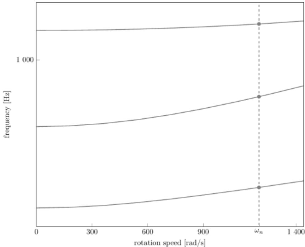
Campbell diagram computed with a linear centrifugal preload, with clamped root (nominal rotation speed  $\omega_n = 1200 \text{ rad/s}$ )
