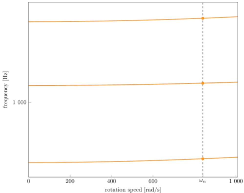
Campbell diagram computed with a linear centrifugal preload, with clamped root (nominal speed  $\omega_n = 839.85$  rad/s),
