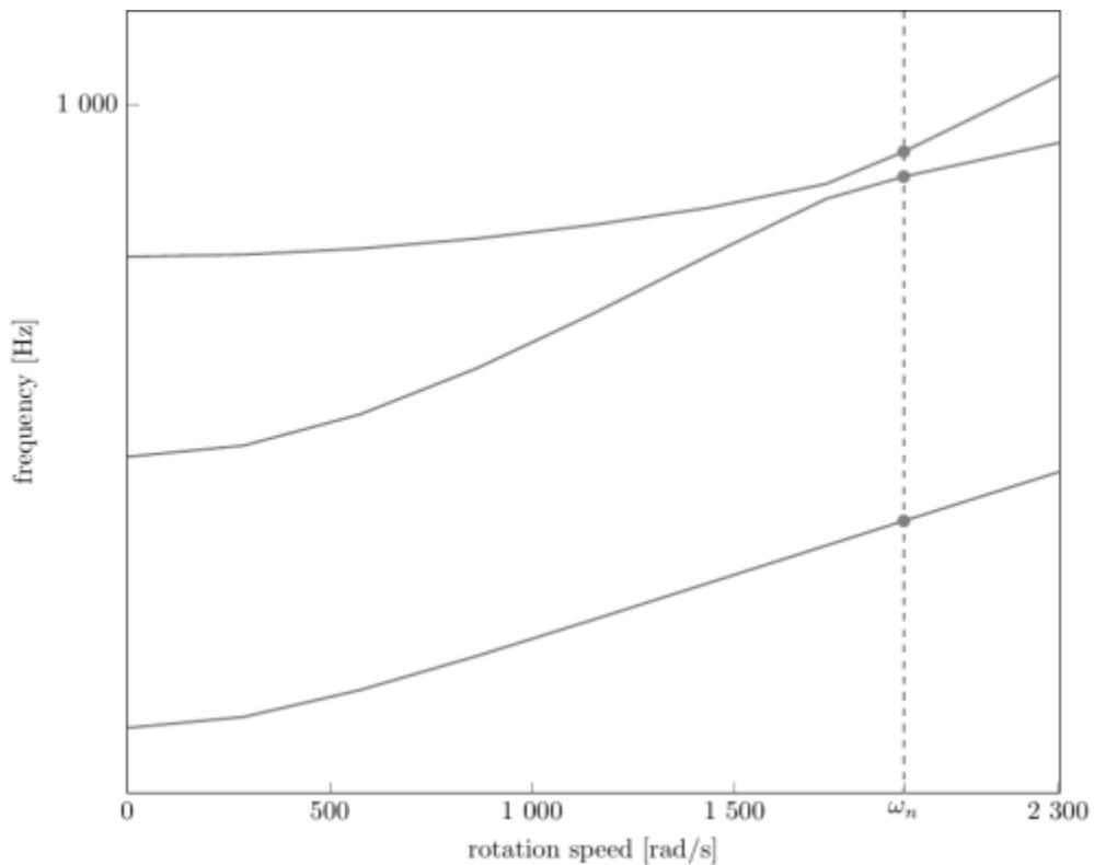
Campbell diagram computed with a linear centrifugal preload, with clamped root (nominal rotation speed  $\omega_n = 1918.66 \text{ rad/s}$ )
