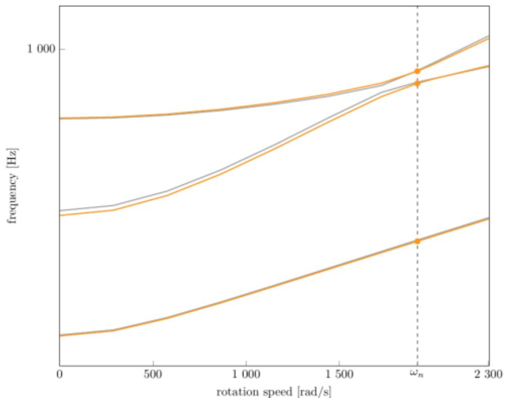
Campbell diagram computed with a linear centrifugal preload, with clamped root (nominal speed  $\omega_n = 1918.66$  rad/s),
