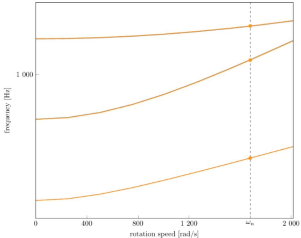
Campbell diagram computed with a linear centrifugal preload, with clamped root (nominal speed  $\omega_n = 1679.94$  rad/s),
