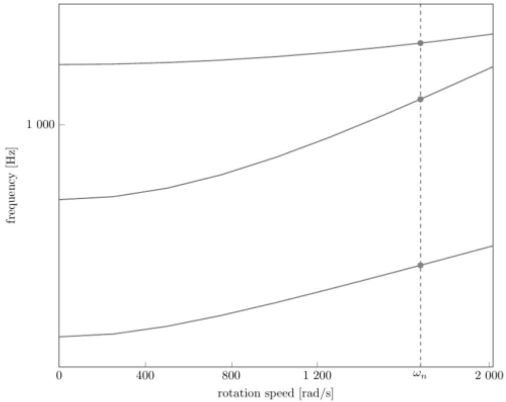
Campbell diagram computed with a linear centrifugal preload, with clamped root (nominal rotation speed  $\omega_n = 1\,679.94 \text{ rad/s}$ )
