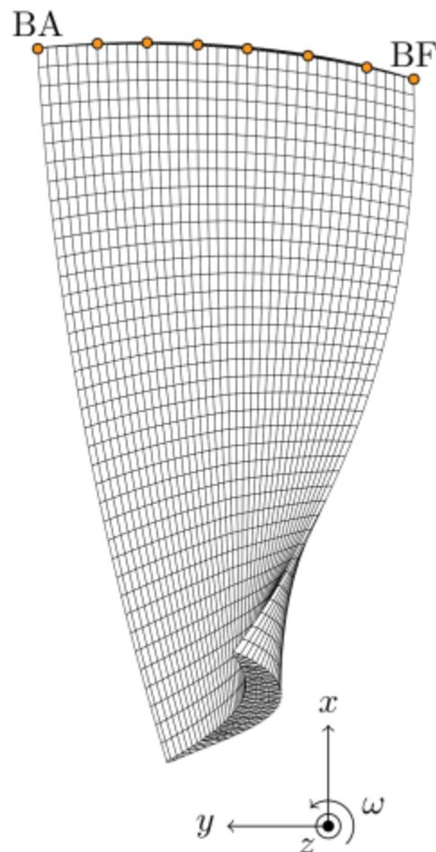
finite element mesh overview (coarse mesh) -
