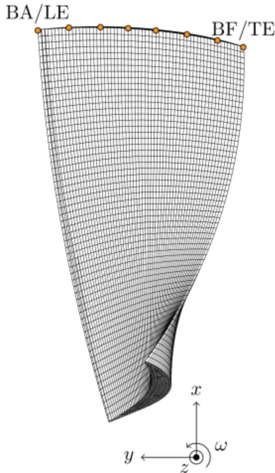
[finite element mesh overview \(refined mesh\) -](#)
