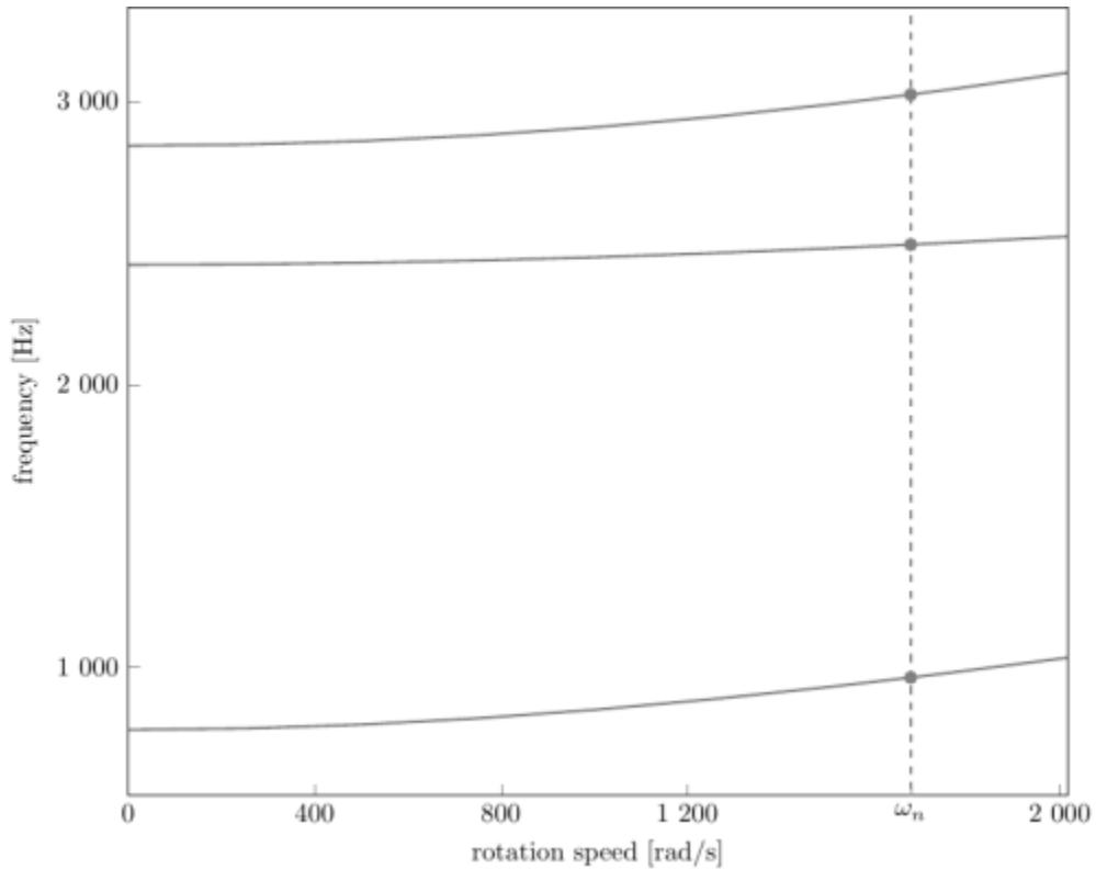
Campbell diagram computed with a linear centrifugal preload, with clamped root (nominal rotation speed  $\omega_n = 1680 \text{ rad/s}$ )
