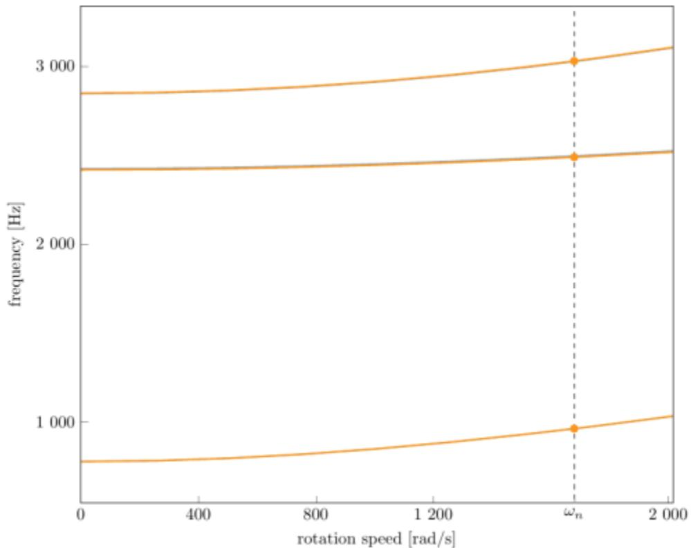
Campbell diagram computed with a linear centrifugal preload, with clamped root (nominal speed  $\omega_n = 1680$  rad/s),
